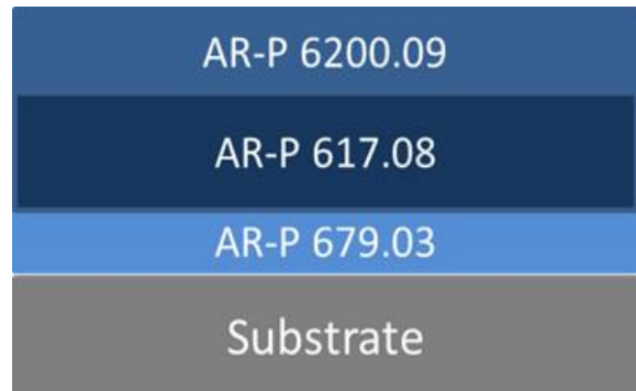
Fig. 10 Three-layer structure of PMMA, PMMAcoMA and CSAR 62
