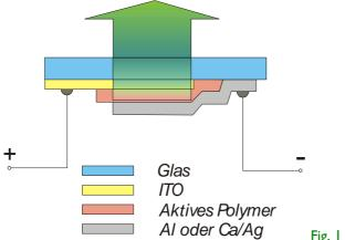
Fig. I Schematic sketch of an OLED
