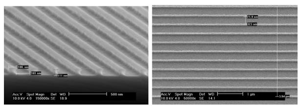
Fig. 8 Photoresist lattice with 300-nm period
