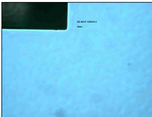
Good resist surface with complete covering of all topologies – positive resist SX AR-P 1250/25.2
