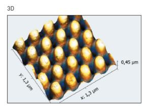
HT-AR-02 surface structures reduce the specular reflectivity from polymer surfaces down to below 0.2%. Our state of the art nano-optical imprinting molds represent the result of years of optical design work and cutting edge origination process development.
